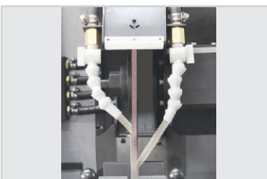
Cut off wheel cooling systems
